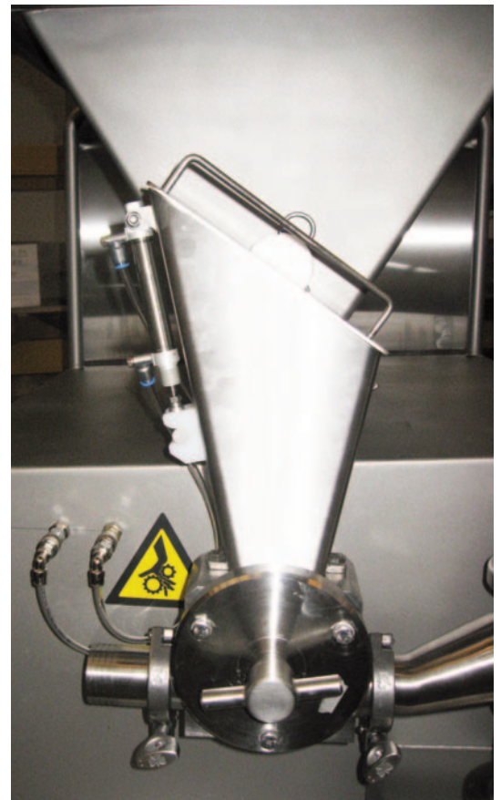
A bridge breaker is available for the Tetra Hoyer Addus fruit feeder
