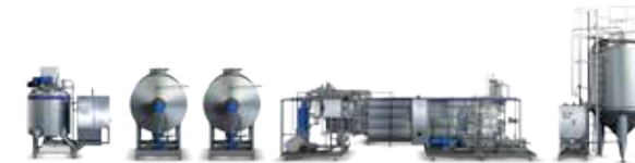
CONTINUOUS LINE For continuous production of smooth to small particulate soups, sauces, desserts, baby food purées, fruit and tomato preparations.
