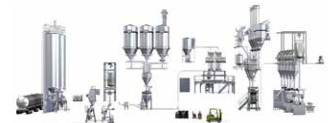
CONTINUOUS INSTANT AND DEHYDRATED LINE For production of instant and dehydrated soups, sauces and bouillons/stocks.
