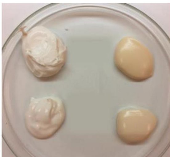
Figure 5. UHT treated spreadable processed cheese samples from a Tetra Pak® Coiled Heat Exchanger (left) and a scraped surface heat exchanger (right) after five months storage at 5°C (lower samples) and 30°C (upper samples).
