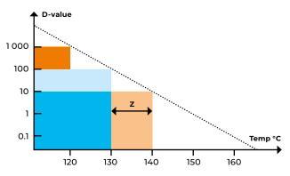
**Fig. 2.** The Z-value is the increase in temperature needed to achieve the same lethal action or the same effect in one-tenth of the time.
