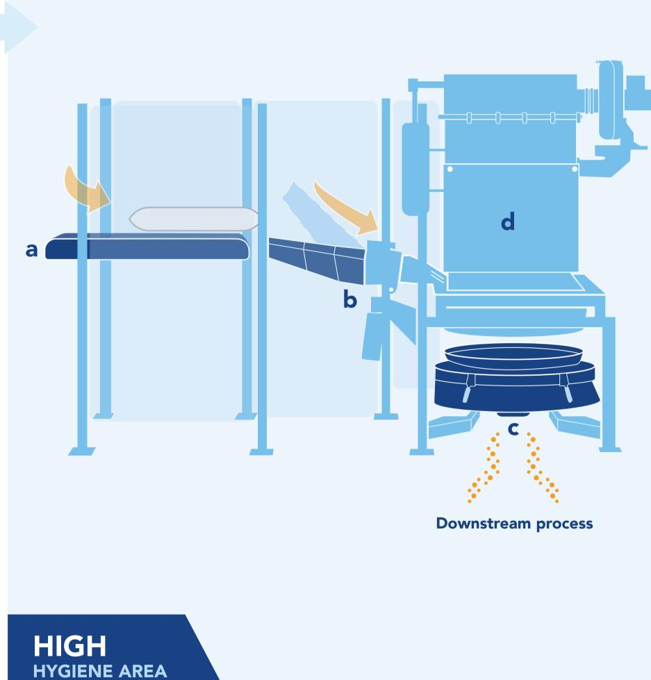
**a.** An **acceleration conveyor** brings the bag forward.
