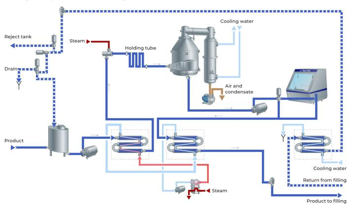
Tetra Pak® Direct UHT unit with infusion and Tetra Pak® Tubular Heat Exchanger with product-to-water heat regeneration.
