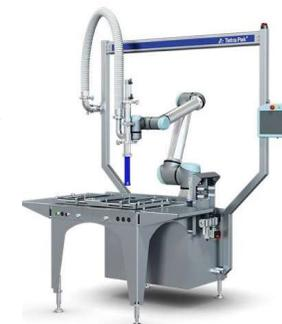
A Cobot is a so-called cooperation robot enabling the machine operator to work with the equipment without the need of separate security dividers, as the equipment will cease production automatically, if it hits the operator. A very convenient security feature!
