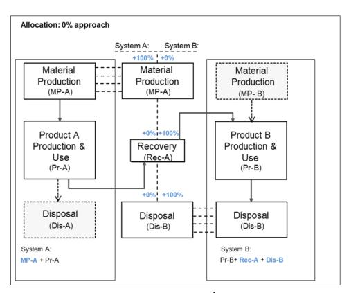
Figure 6: Principles of 0% allocation (schematic flow chart)<sup>1</sup>
