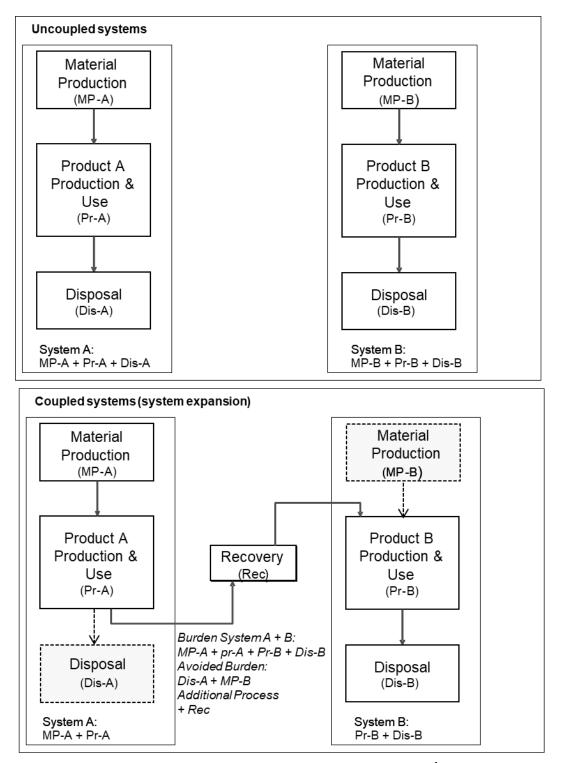
Figure 3: Additional system benefit/burden through recycling (schematic flow chart)<sup>1</sup>
