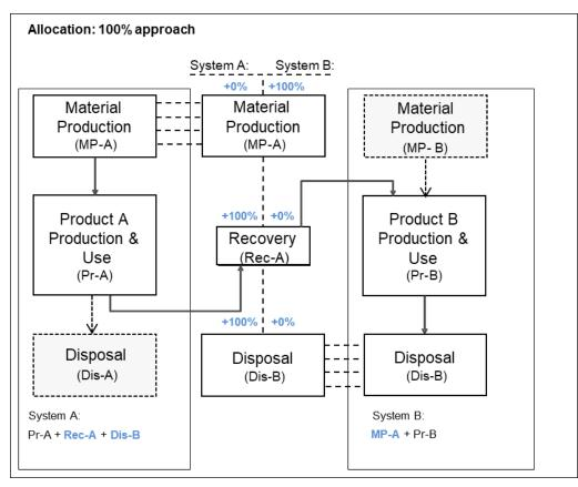
Figure 5: Principles of 100% allocation (schematic flow chart)<sup>1</sup>
