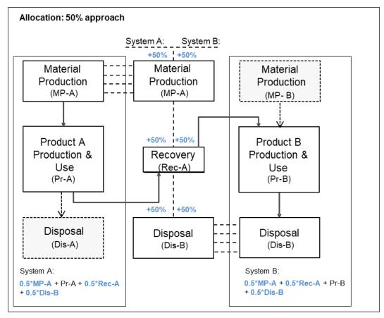
Figure 4: Principles of 50% allocation (schematic flow chart)<sup>1</sup>
